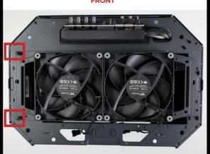
BACK Disconnect any fan cables as needed to fully remove the top fan bracket.
